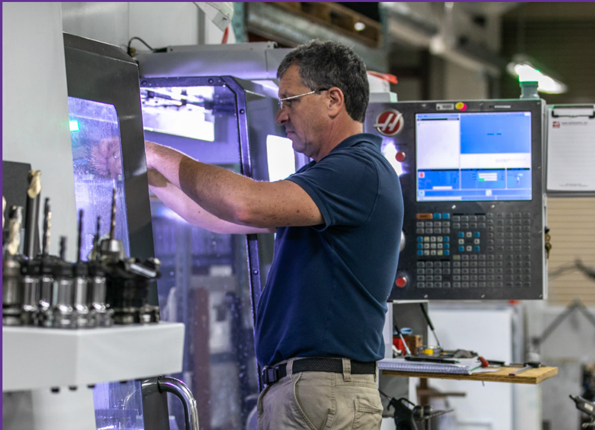
Tim Evans, a mechanical engineering technician, uses a computer numerical control machine to machine a part for a Launch Pad 39B camera enclosure inside the Prototype Development Laboratory at NASA's Kennedy Space Center.
